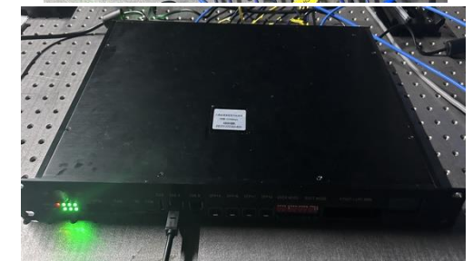
Bunch by bunch profile monitor prototype: photodetector, DAQ
